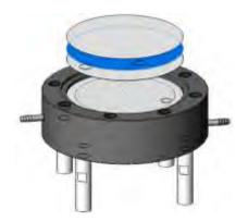
Place the desired size of nanometer membrane carefully on the stainless steel micron pore of the support plate (3).
