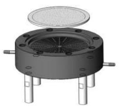
Install the stainless steel micron pore support plate (3) on the filter support base (2).
