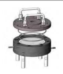
Install the small O-ring (4), large O-ring (5) and the gland (6) on the filter support base (2) in order.
