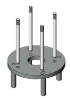
Mount four pull rods (11) on the bracket base (1).
