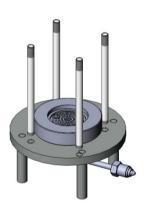
Place the mounted units in step 3 onto the bracket base (1).
