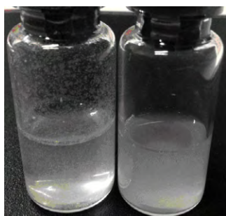
图 6 喜树碱原粉 (左) 和喜树碱微粉 (右) 在水中的分散性 Fig. 6 Dispersion appearances of raw CPT (left) and CPT micronized powder (right) in water
